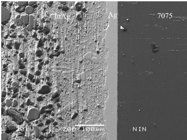
Fig.3 The SEM image of In-7Ag welded joint
